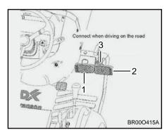
(1) Brake Pedal (L) (2) Brake Pedal (R) (3) Brake Pedal Coupler
