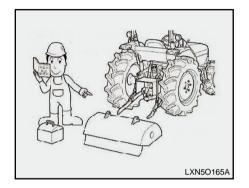
Move wheels to widest setting when working slope or when towing.
