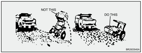
When transporting the load, keep the bucket as low as possible to avoid tipping, in case a wheel drops in a rut.
