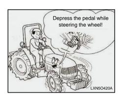
When making a turn, reduce the engine rpm and make a slow turn. When making a turn on the pavement, remove the connector of the brake pedals. Depress the brake pedal on the side to which to make a turn, while steering the wheel, this will allow the tractor to make the turn without moving ahead. Make sure to keep the implement in the up position when making a turn.
