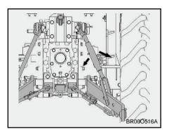
4. Level a 3 point mounted implement from side to side by turning the adjusting handle to shorten or lengthen the adjustable lifting rod with the implement on the ground.
