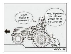
Enter or leave the pavement in a perpendicular direction. When climbing onto the pavement, lower the implement to achieve a lower center of gravity. Once all wheels of the tractor are on the pavement, raise the implement.
