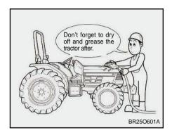
After work, clean the tractor, After cleaning, dry the moisture and supply grease into each grease nipple. Avoid water on electrical parts whenever possible, as it will cause equip-
