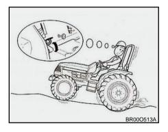
Depressing the differential gear lock pedal will make both rear wheels roll
