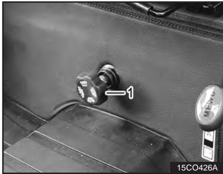
(1) Flow Control Valve
