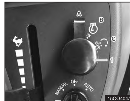
(1) Main Key Switch
